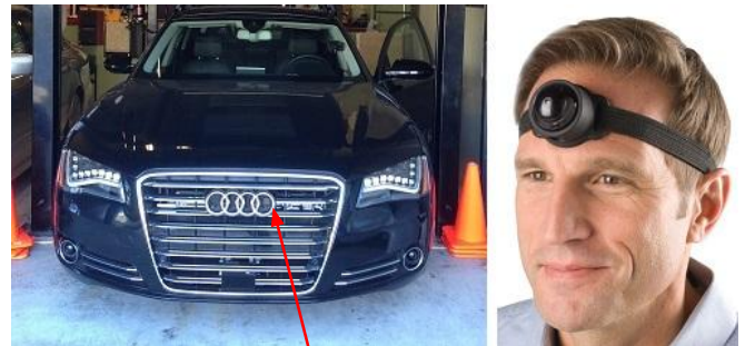
Fig. 1. Left and right images show the positions of two cameras. The external camera is located in front of a car and the internal camera is mounted on a driver’s head.
